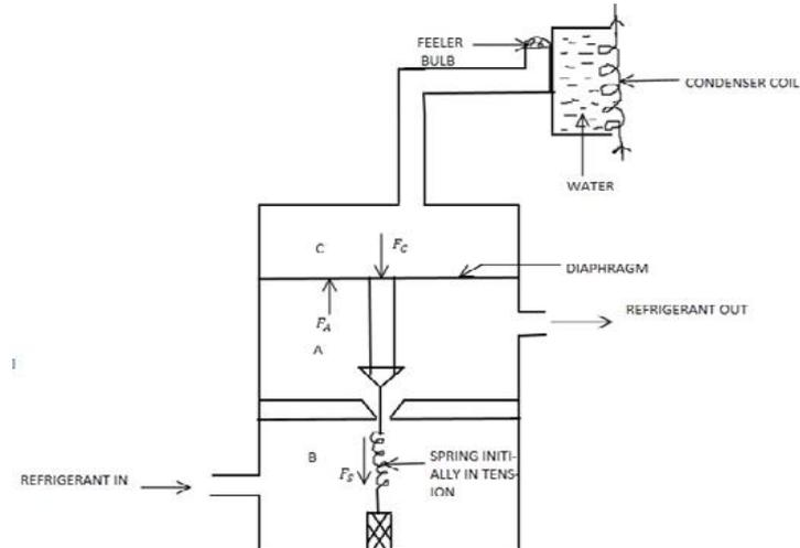
**Figure 3: Thermostatic Valve**
