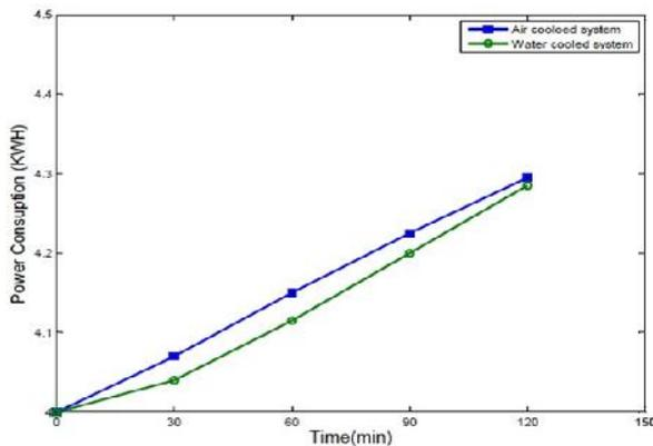
Graph between energy consumption with Air cooled and Water cooled Condenser of Refrigerator Vs Time
