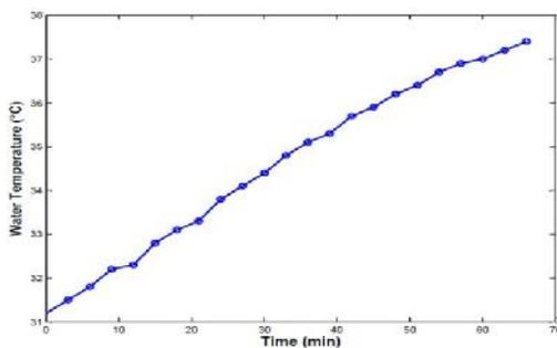
Graph between water temperature Vs time (when the water cooled condenser are open)
