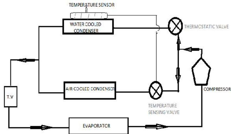
**Figure 5: Heat Recovery in Domestic Refrigerator Using Two Condensers**
